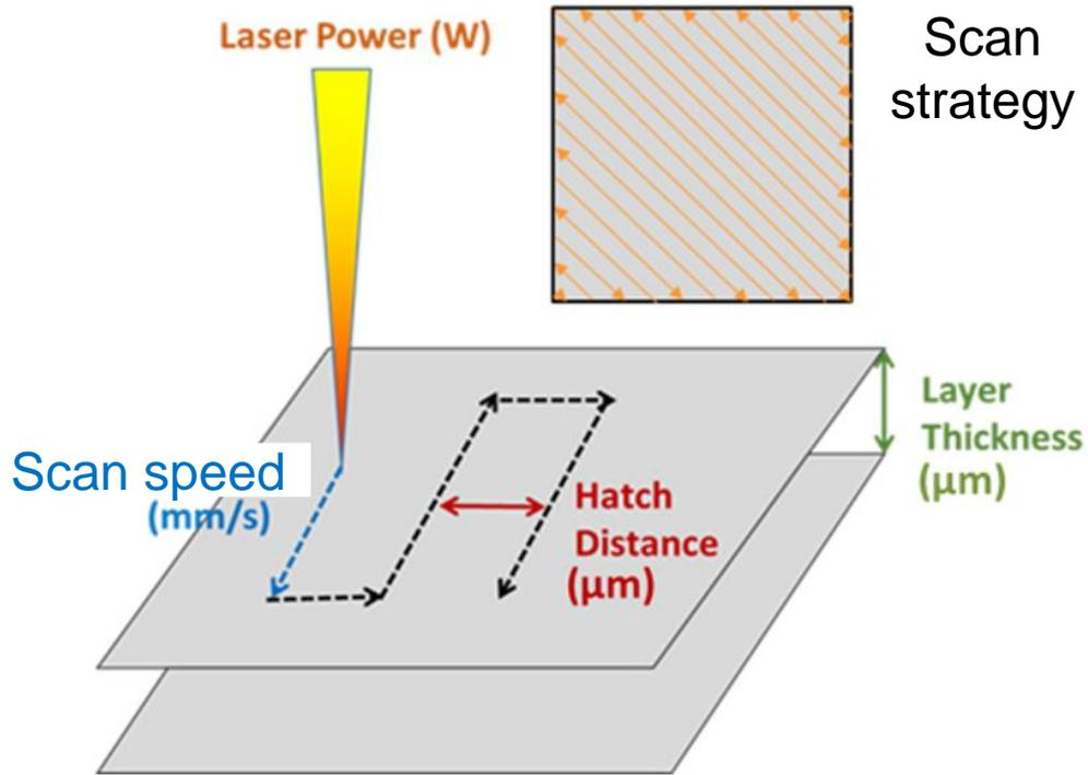
Fig. Common process parameters
