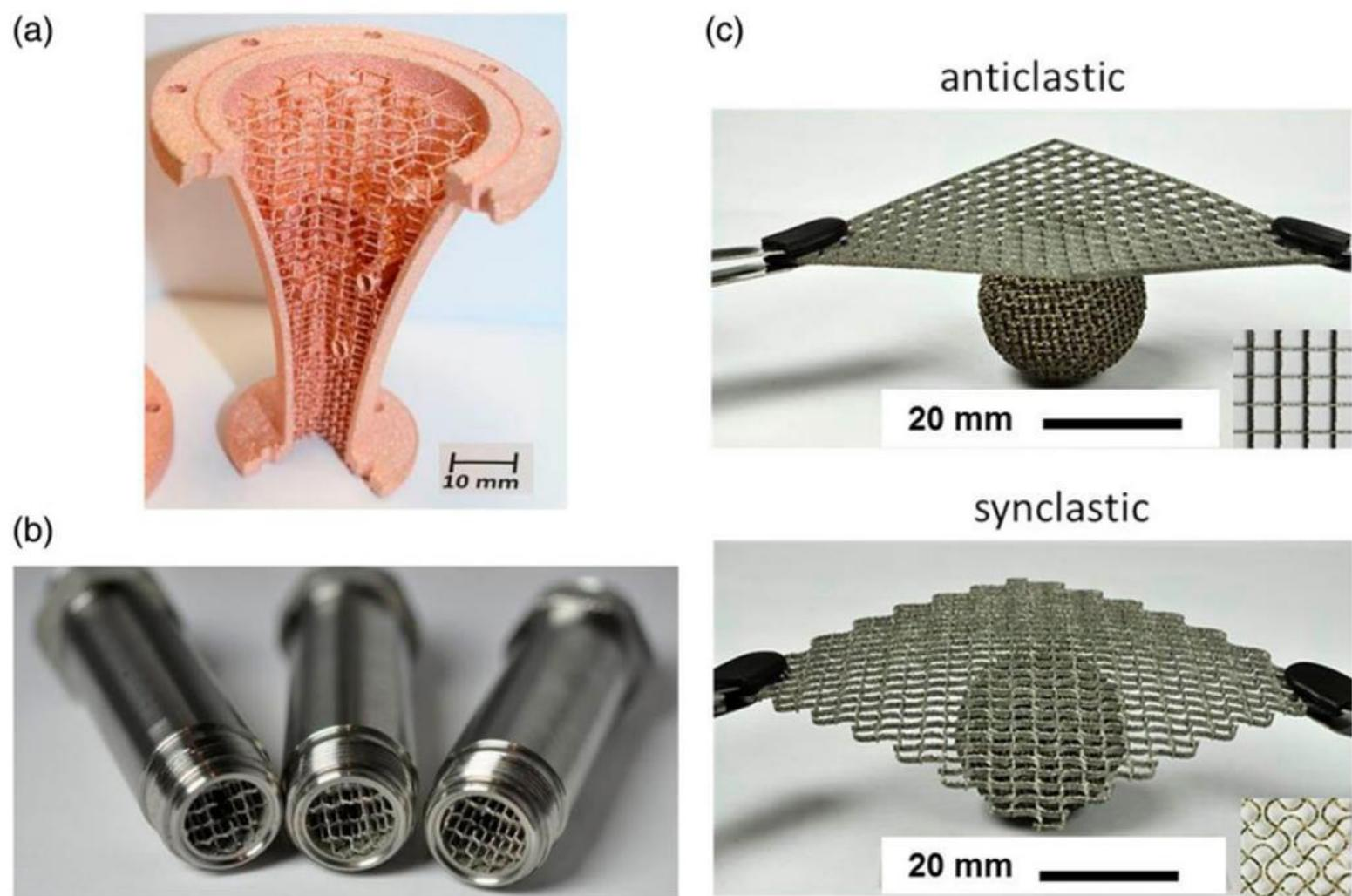
**Fig.** Cellular structures and materials: (a) pure copper component with a cellular core, (b) SS reactor for hydrogen release from perhydro-N-ethylcarbazole, and (c) Ti-6Al-4V lattice structure (anticlastic) versus auxetic structure (synclastic)
