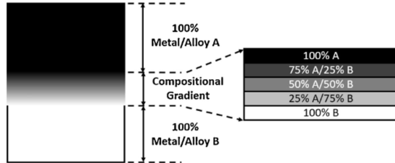
**Fig.** Schematic illustration of FGM comprising metal/alloy A, and metal/alloy B.
