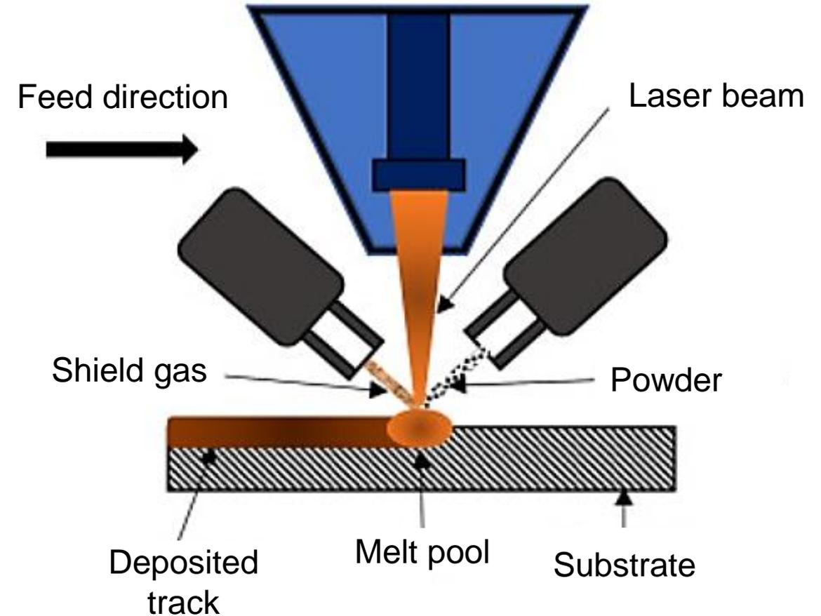
**Fig.** Schematic Laser Metal Deposition (LMD) process
