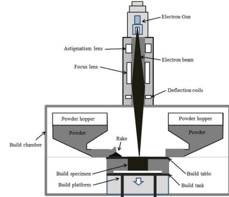
**Fig.** Schematic principle of Electron Beam Melting (EBM)
