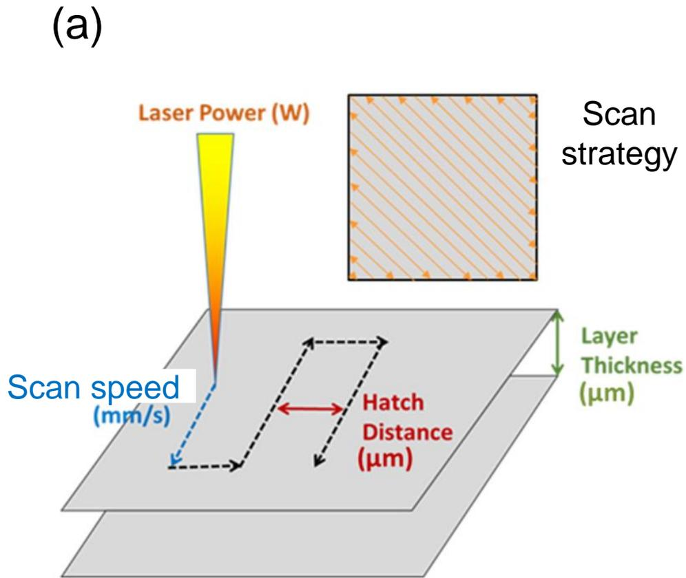
**Fig.** Common LPBF process parameters
