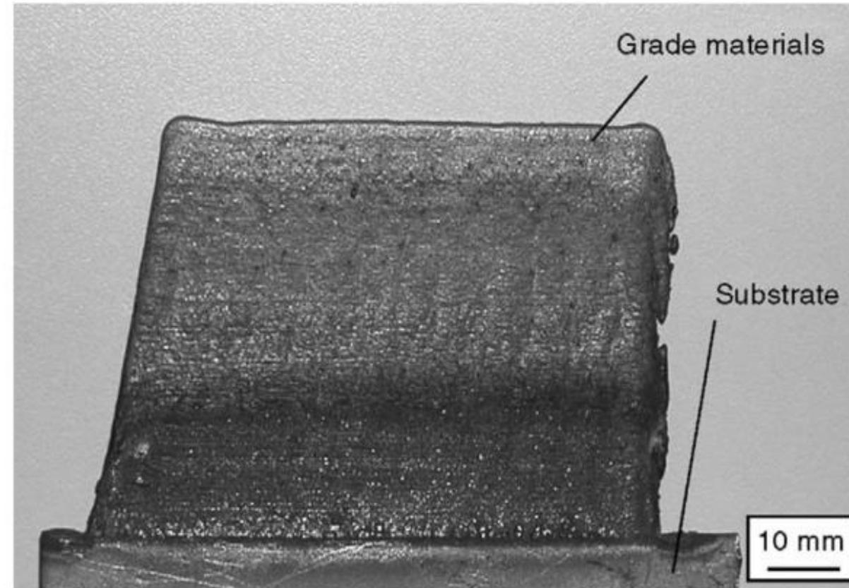
**Fig.** LMD build SS316L/Rene88DT FGM on SS316L substrate
