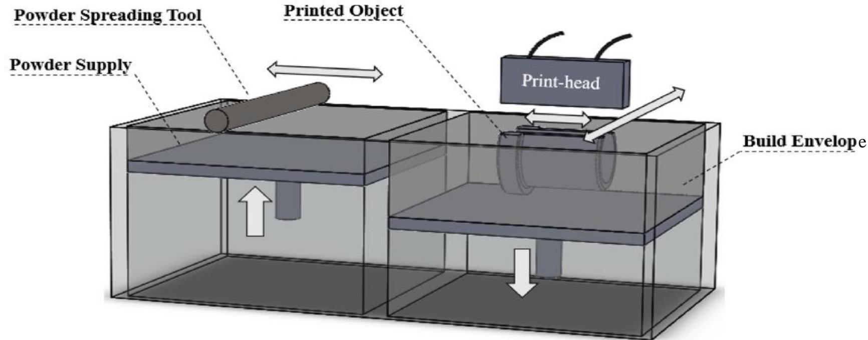
**Fig.** A schematic binder jetting system
