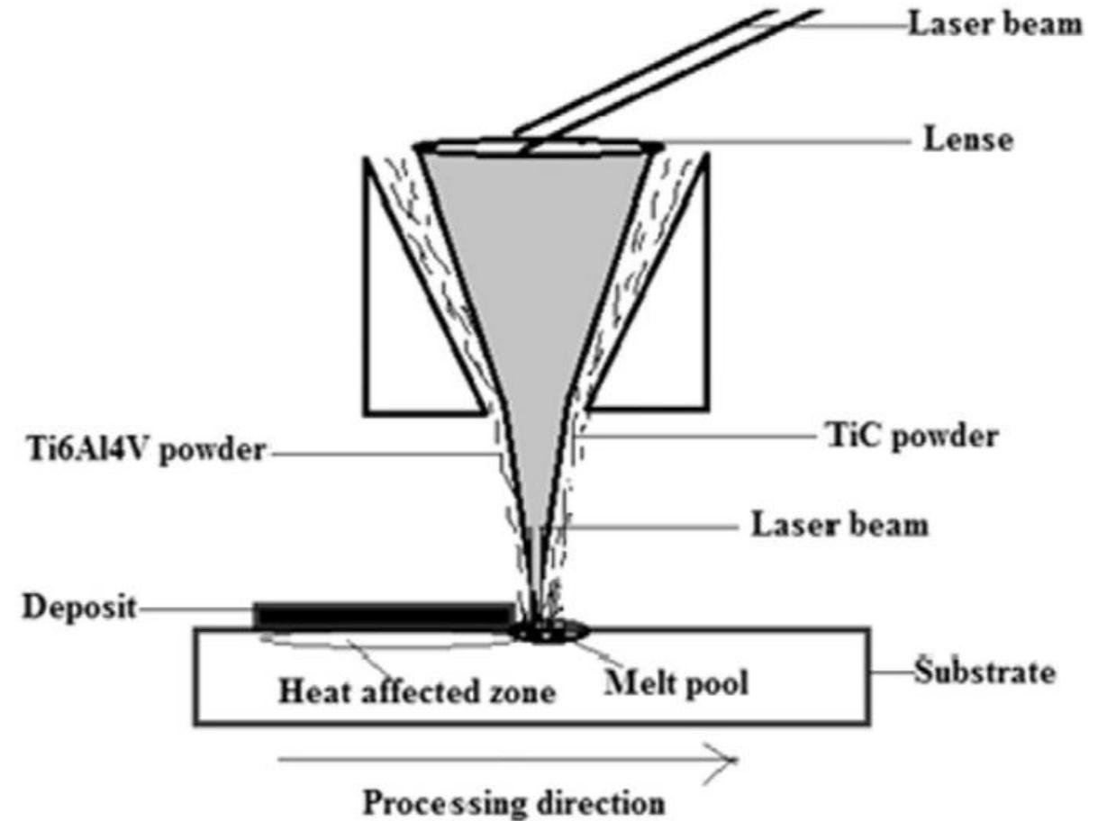
**Fig.** Schematic Laser Metal Deposition (LMD) process for FGM
