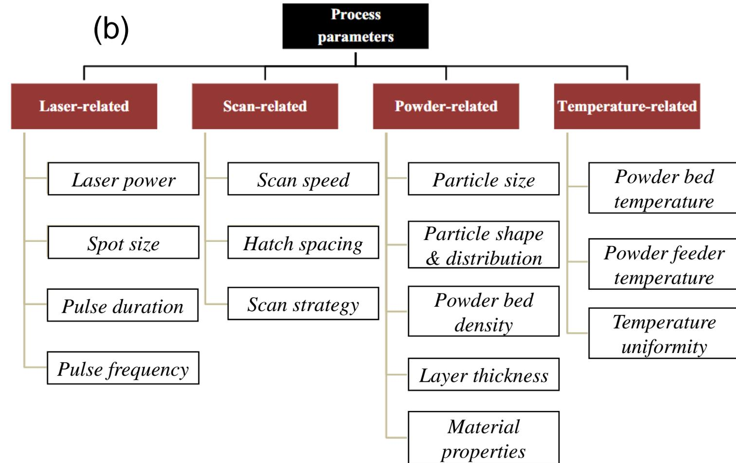
**Fig.** Classification of LPBF process parameters
