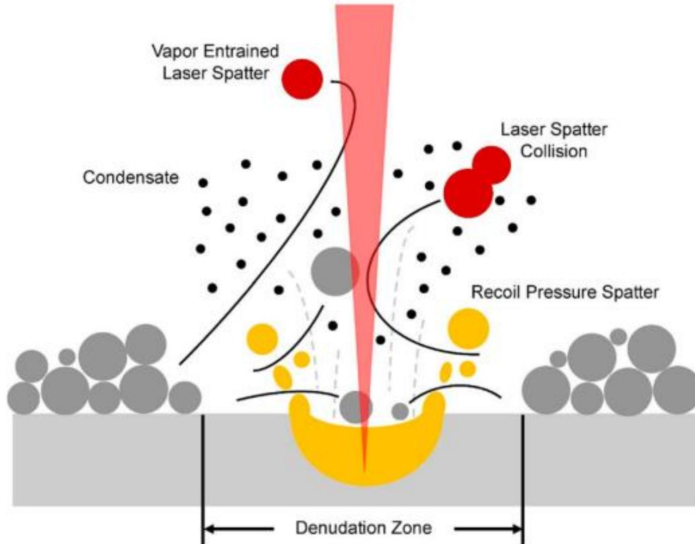
**Fig.** Laser spatter and condensate formation during LPBF
