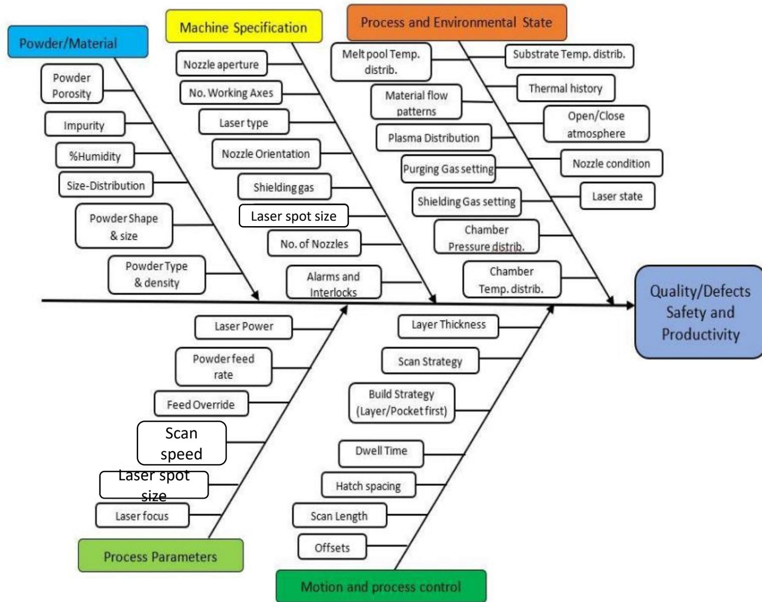
**Fig.** Process/material parameters in LMD process
