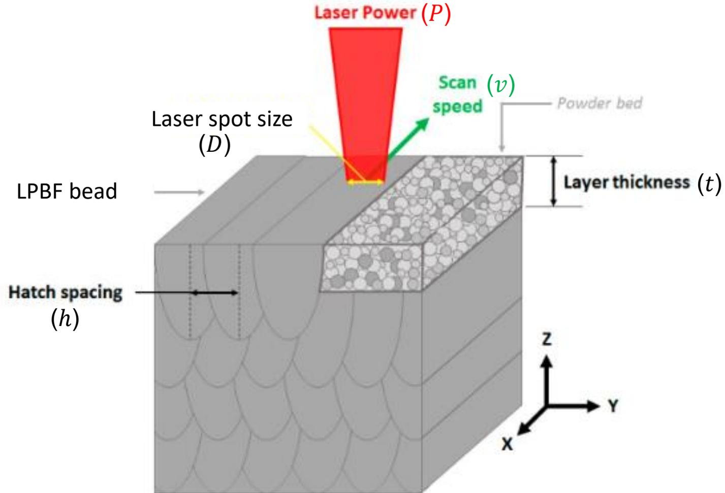
**Fig.** Schematic illustration of Laser Powder Bed Fusion parameters
