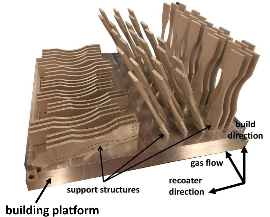
**Fig.** LPBF built specimens on a build plate
